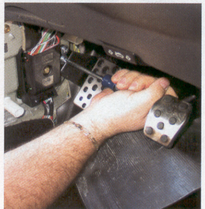
Two self-tapping sheetmetal screws are included with the pedal. Simply screw them in to secure the pedal.
