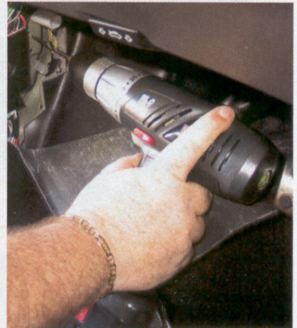
After moving the carpet out of the way and trimming the insulation, use the pedal's bracket as a template to mark the sheetmetal. Then use a \frac{3}{16} -inch drill bit to carefully drill through the inner sheetmetal panel. Don't get too deep and drill through the side of your Focus!
