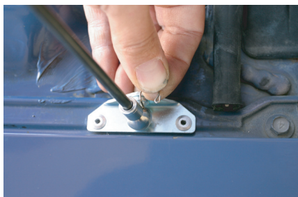
Insert clip into hole.
