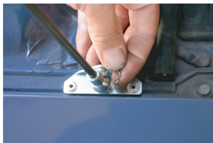
Slide clip down till it stops.
