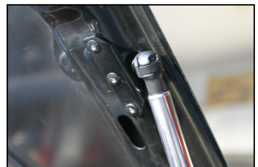
C. Slide clip over ball-stud to lock end-fitting
